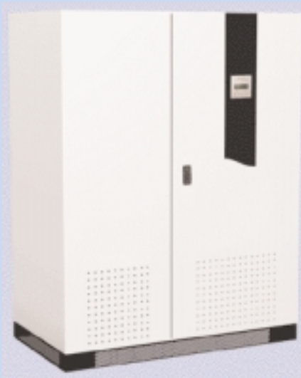
Distribution and protection of single-phase electronic equipment. Rated supply 250 A three-phase. Two versions for 60 outgoing circuits (16 A) with earth-leakage protection or 126 outgoing circuits (16 A) with thermal-magnetic protection. Optional built-in transformer.
