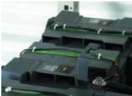
Reduced cabling: 1 wire per block
